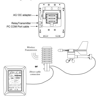
Independently of the final power supply mode, the fixed cable of the Wind Sensor has first to be connected to the Relay Transmitter by plugging it into the marked receptacle.
