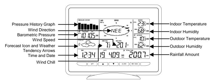
Press the SET key to toggle between Mode 1 and Mode 2 display:
