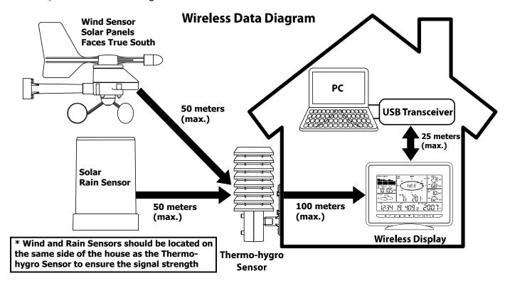
The thermo-hygro sensor measures outdoor temperature & humidity and collects the data from the wind and the rain sensors and sends all outdoor weather data to the wireless display, so the thermo-hygro sensor must be within the 100 meters wireless range of the wireless display. This allows the wind and rain sensors to be placed relative to the thermo-hygro sensor rather than the wireless display. See Wireless Data Diagram above.
