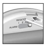
If the clock behaves strangely or stops responding, insert and press a blunt stylus into the vibration device's Reset Hole. (This is located inside the vibration device. Remove the back of the vibration device just above the Alarm 1, Alarm 2, All switch and above the battery compartment).
