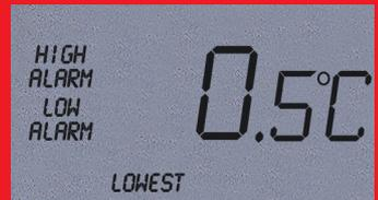
LCD displays lowest recorded reading
